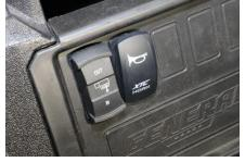
Connect to OEM Dash Indicators - Note: The connector has power in it, disconnect the battery during installation. There is a 2-wire harness that has green and yellow wires coming out of it. The Ranger uses the green and yellow wires to light the Arrows in the OEM instrument cluster.
