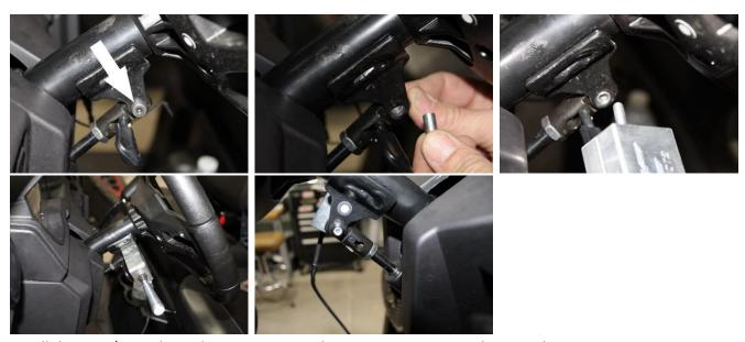
7. Install the Horn/Hazard Switches. Using a new sharp razor, cut one switch rectangles out. Do not over cut, try inserting switch and trim as necessary. It helps to rock the razor to cut. Run Switch Harness – Plug the Switch Harness into the Control Module, run the connectors through the rectangle switch cutouts and use included grease on switch terminals, then connect and slide switch into dash.
